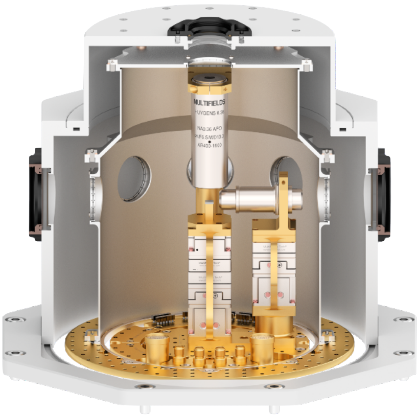
Figure 1. Configuration of Optical Waveguide Excitation Experiment on ColdTABLE.
