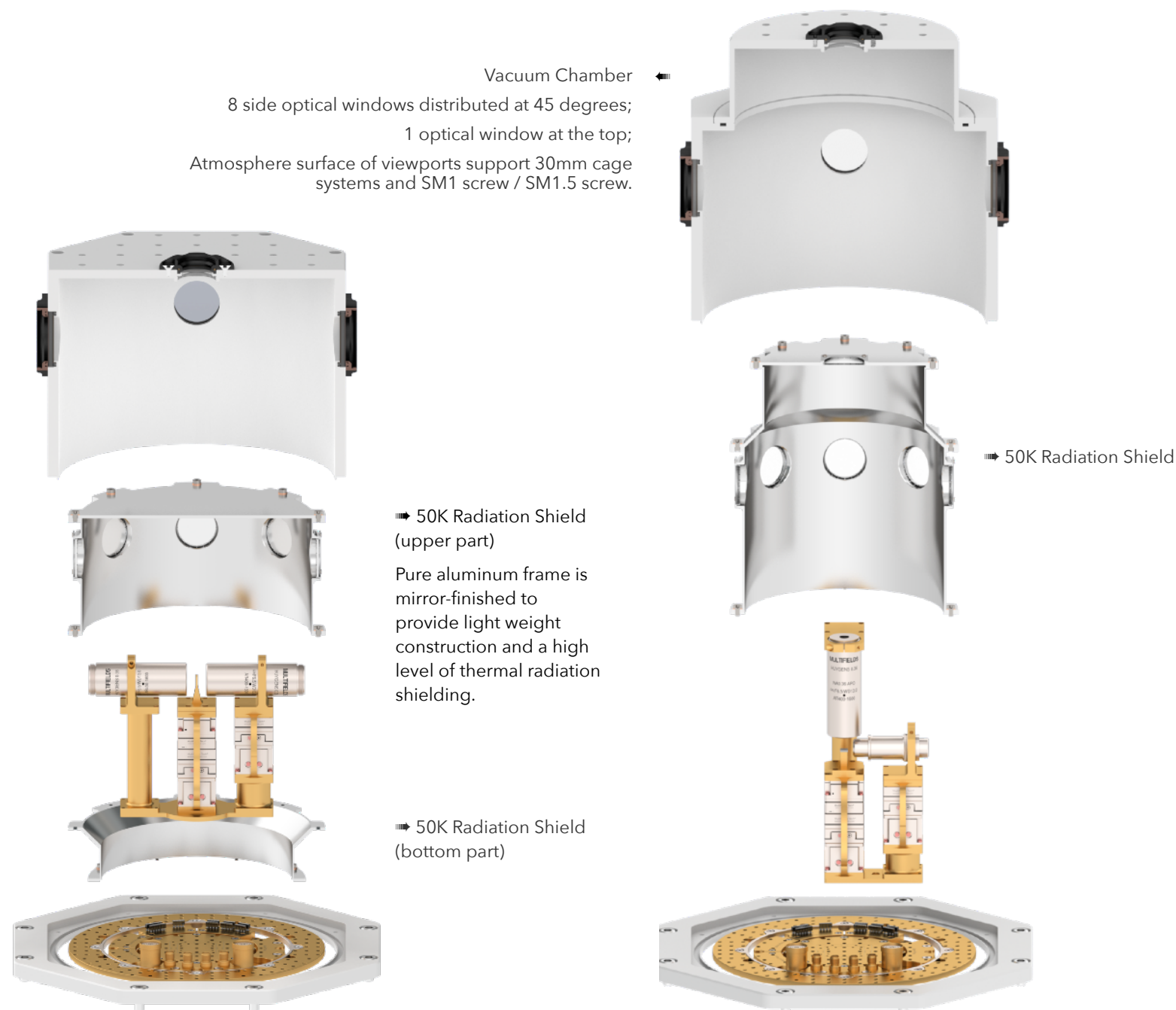
Figure 1. Schematic of transmission experiment with customized radiation shield and vacuum chamber.
