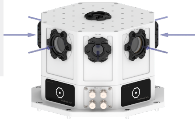
Figure 1. Optic access to sample chamber, schematic of windows spatial configuration.
